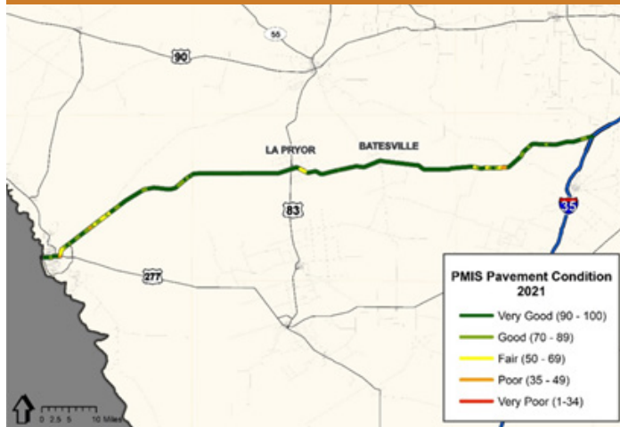
Figure 6.20 - US 57 Pavement Condition
